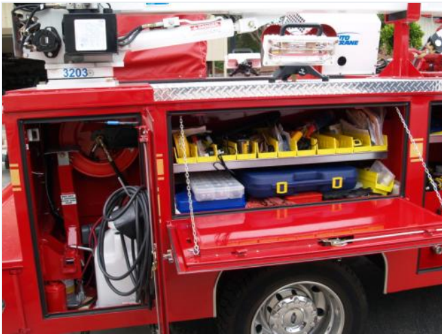
Jacks, absorbent, Air reel, more parts and crane controls
