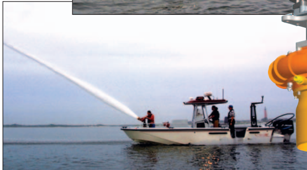
The Darley PSE Pump coupled to the Mercury 200 HP outboard marine engine delivers flows over 1500 GPM.
